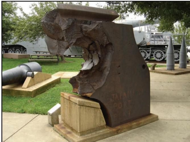
thick steel plate that would have been used on a Japanese *Yamato* class battleship. After the war, the US Navy conducted ballistic tests using a standard 16 inch naval gun. Well, the above photo speaks for itself!
