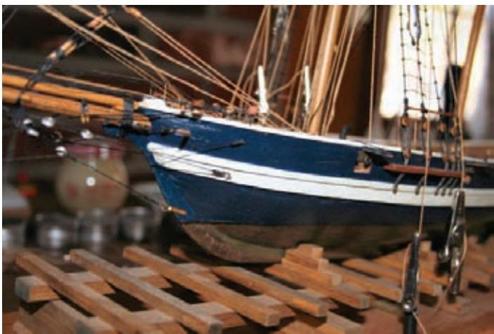
pleted and current projects. The "Model Shipways" kit of the Baltimore Clipper *Dapper Tom* (above) was converted from solid hull to plank-on-bulkhead, making it practically a scratch-built model.
