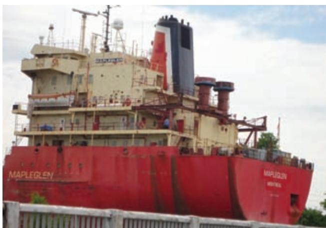
paint, a type of protective primer. Also, the forward part of the bridge indicates that the peeling paint has been removed from the port side, and a grey primer, or new color, has been applied. So, it would seem that some efforts are being made to spiff up the 51 year old ship.
