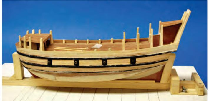
Another use of the wood filler was in creating treenails in the deck. Holes were first drilled using a spacer jig and then filled with wood filler. The result looks very authentic.
