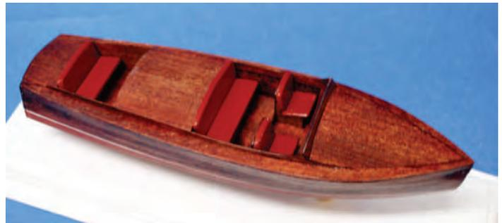
any furnished with the kit needed a lot of work sanding and shaping in an effort to achieve a good finish. The seats are made of balsa with eight coats of primer, paint and lacquer. Lower hull color is GM 1965 Flame Red - matches Chris Craft perfectly.
