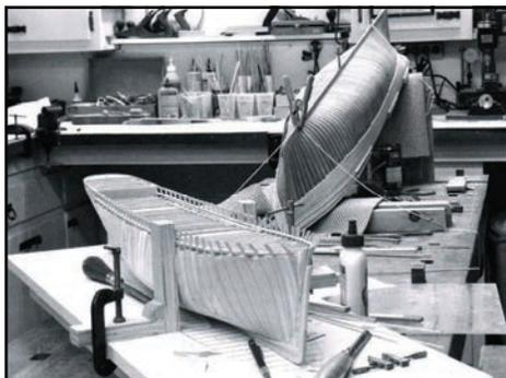
plank on bulkhead model of the *Young America*. Even at this smaller scale, the hull measures a very impressive 40" in length.
