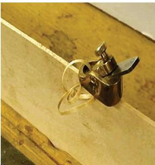
Shavings are created using a finger plane cutting wood stock of a thickness equal to the desired width of the finished mast hoop. The shavings are made thin enough to allow curling around a dowel and gluing to complete a hoop (per photo #2).
