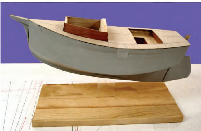
to contend with trying to position the R/C controls in such a way that the boat floats on an even keel. A drop center board will be added to give the necessary stability to the mast and sail and will replace the display pylon shown in clear plastic.
