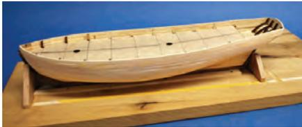
**Ray Oswald's** ship's boat was built over a plug that was mounted on a building board with station lines drawn on it and removable blocks to hold the plug firmly in place.
