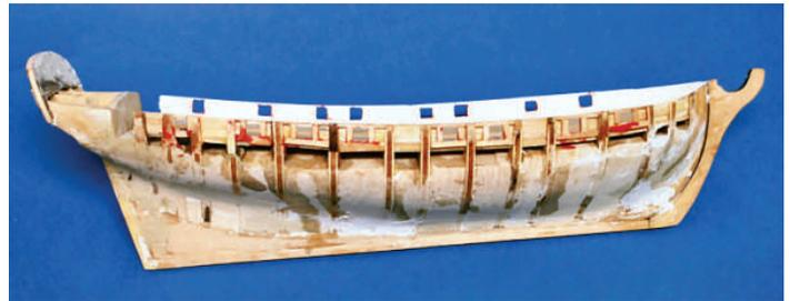
Here we can see Sid's building method of planking from the inside out. The inboard bulwarks have been fully planked and primed and the gun port openings have been framed and painted. Now all that remains is to plank the outer hull. Looks like a great building technique, mate.
