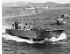
designed for carrying vehicles. They were used to land troops or tanks. The LCM (2) was the first American design with approximately 150 built by American Car & Foundry and Higgins Industries. Higgins built the LCM (3), which was capable of carrying 120,000 lb of cargo. Other variants were built by the UK.
