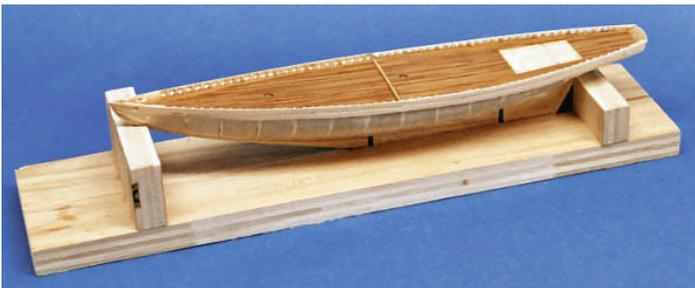
the fishing schooner *Blue-nose*. Using "Model Shipways" plans, he reduced the scale 50% to arrive at the size model he wanted. Decks were re-planked over balsa and bass wood fillers between bulkheads to eliminate "sponginess" caused by a lack of support for the planks. The next challenge for Ken will be to cut out scuppers in the bulwarks - not an easy job at that scale.
