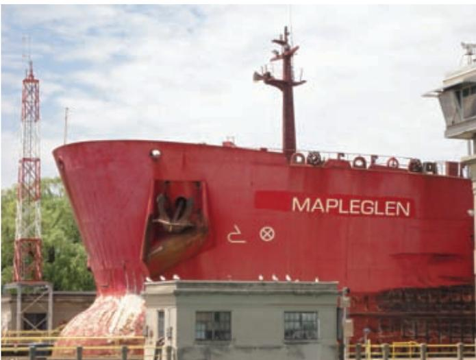
Capable of over 13 knots, this 17,000 ton vessel has a length of 715 feet, and can carry over 26,000 tons of cargo for a maximum draft of 27 feet.
