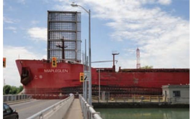
If you look closely at the above photo, the ship is riding high, and the internal hull framing is quite evident where the hull plating has been pushed in. This vessel definitely shows signs of a long, hard career!
