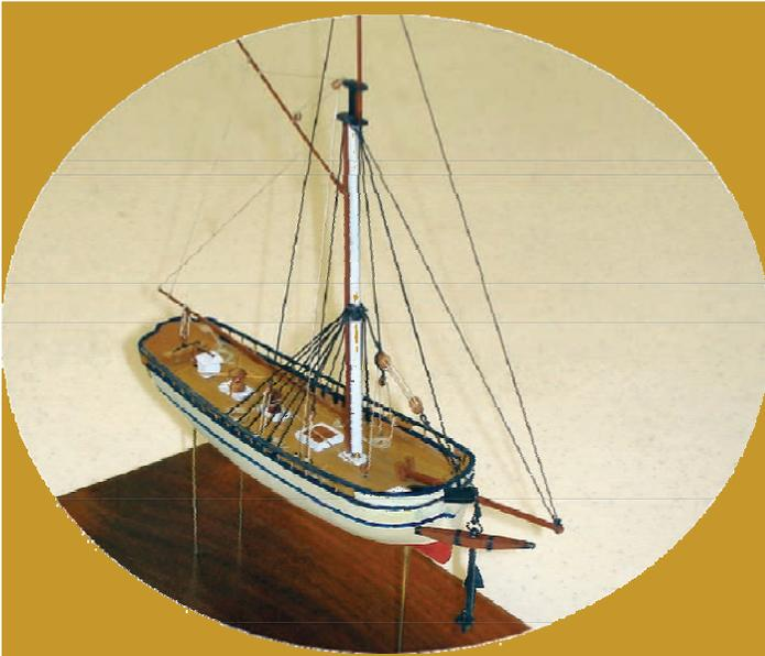
main mast is a Spencer mast to handle the fore-and-aft main sail boom and gaff. Heavy capstan gears in the stern allowed the bow to have additional flotation to offset the weight of the suspended anchor.
