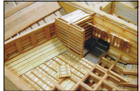
Chapters 23 through 29 discuss the orlop deck and hold, aft platform and magazine, deck beams, knees, the lower deck framing, and the wale and related work. The author's description for laying out the large deck beams is particularly interesting, since it involves short sections scarphed together with long tabled joints. Apparently, this was quite common as larger lumber became harder to come by in
