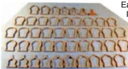
Each sheet was then hollowed out to the inner hull shape before being glued back together. Lower hull frame spacing was created by cutting off frame sections.
