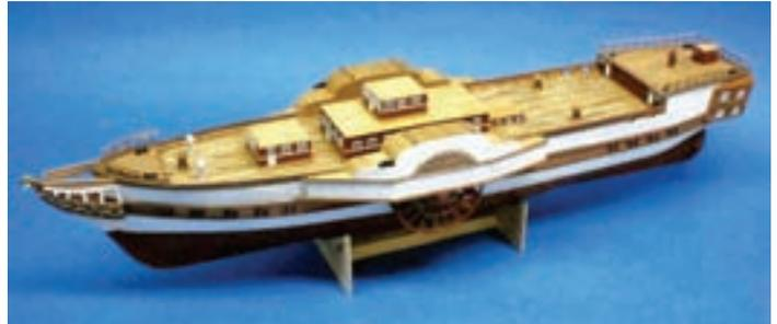
This is a very unusual type of vessel, having both steam driven paddlewheel as well as sail propulsion. The ship
